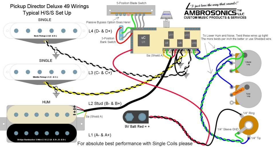
use 2-Conductor + a Shield wire with one end of the braided Shield connected to Sa (Shield a) or Sb (Shield b) at the Pickup Director PCB and left open at the Pickup end.
