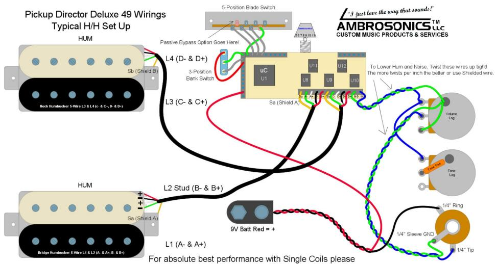
use 2-Conductor + a Shield wire with one end of the braided Shield connected to Sa (Shield a) or Sb (Shield b) at the Pickup Director PCB and left open at the Pickup end.
