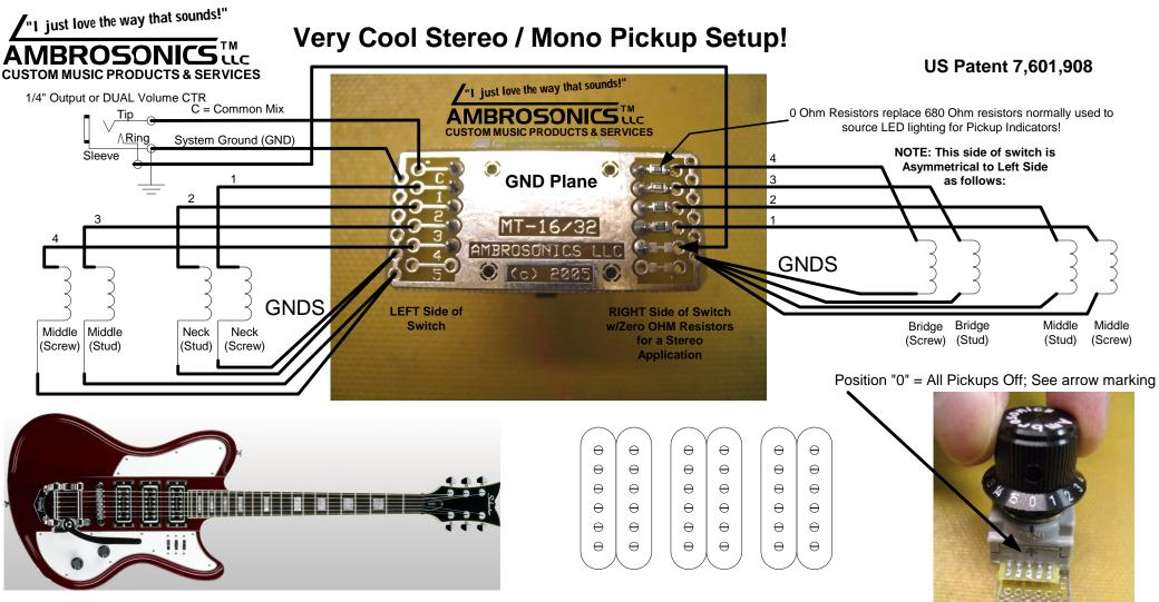
One Switch Provides the switch closures shown in the chart below X 2! (Left side & Right side of switch for Stereo Mode)
