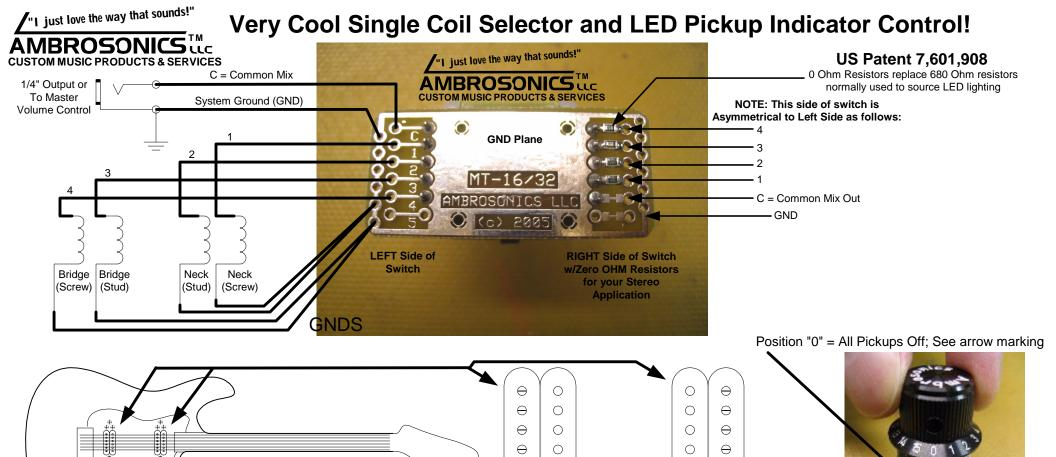
One Switch Provides the switch closures shown in the chart below X 2! (Left side & Right side of switch)
